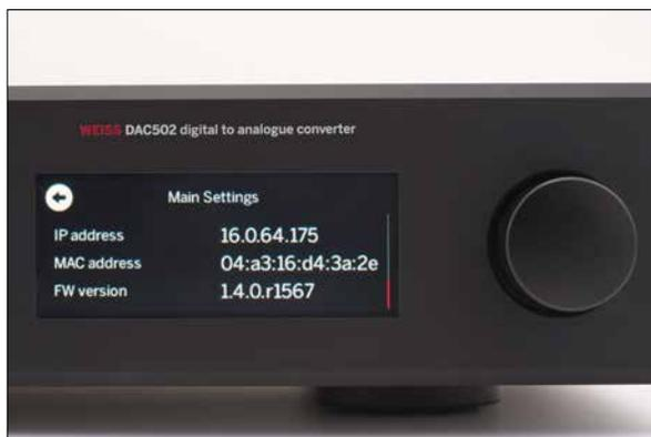
◀ In the “Main Settings” menu, basic configurations can be set such as choosing between four (analog) output levels.
